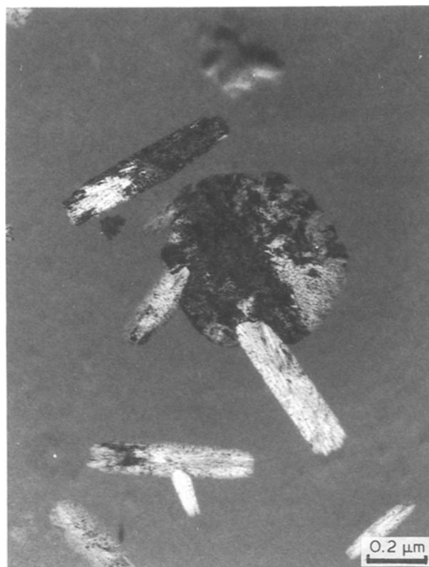
Figure 1 Bright-field TEM image of film evaporated at 370^\circ\text{C} for 10 min. The thickness was 55 nm. Spherulitic and rectangular metastable crystals are observed.
